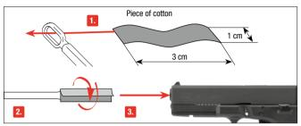
Prepare a thin rod with a length of approx. 30 cm. Attach a piece of cotton fabric to its end and clean the barrel with some silicone oil
